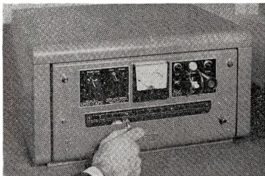
Gates spot selector contains tape belt inside above unit
